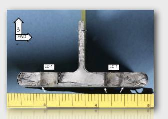
International Airport (DAB). A second ERAU Piper was found to have a similar fatigue crack in its left-wing main spar when the school's fleet was examined after the accident. The board noted that no anomalies in materials or construction of the wing spars were found on either aircraft.
